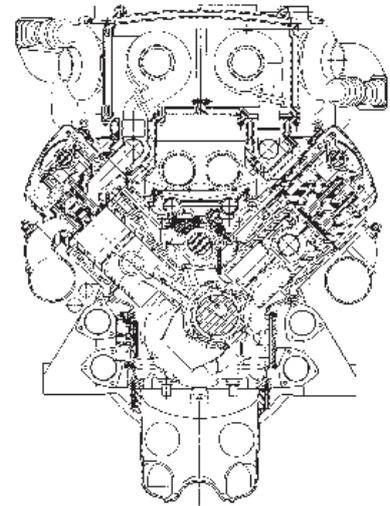
engine block. The liner is trapped between the crankcase and the cylinder head at the liner flange. The lower support for the liner is arranged to be high in the crankcase and incorporates two 'O' ring seals and a large 'wedge' ring.
